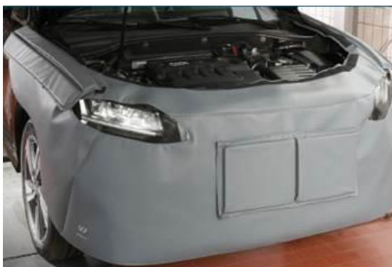
Figure 3. Protective workshop cover.
