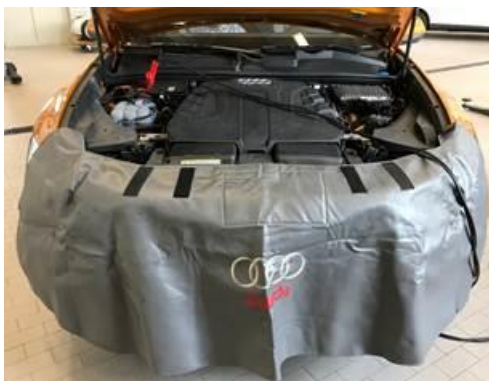
Figure 2. Protective workshop cover.
