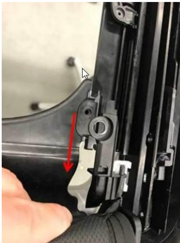
Figure 4. Slide roller shade backward.
