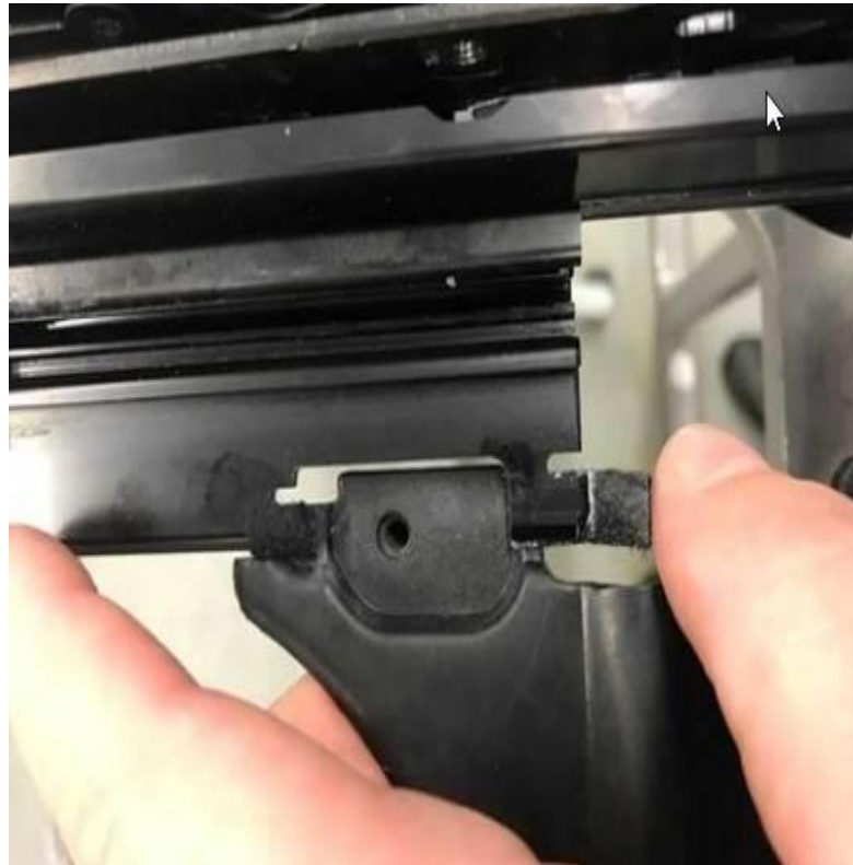
Figure 6. Applying felt tape.
