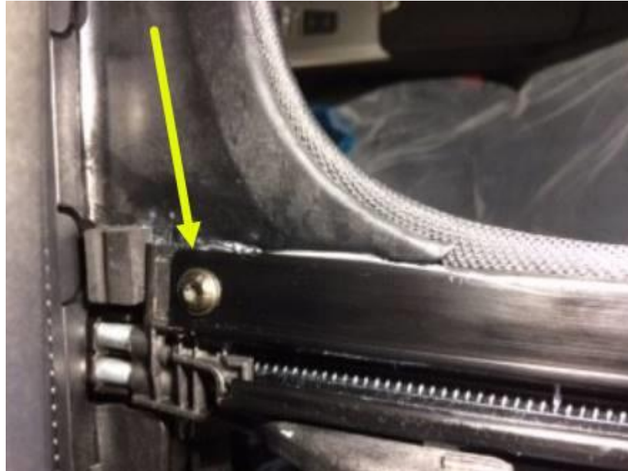
Figure 8. Loosen bolt and apply lube paste between these panels and under the bolt head. Reinstall bolt and torque to 5Nm.
