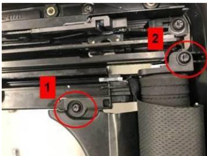
Figure 3. Remove the bolts.
