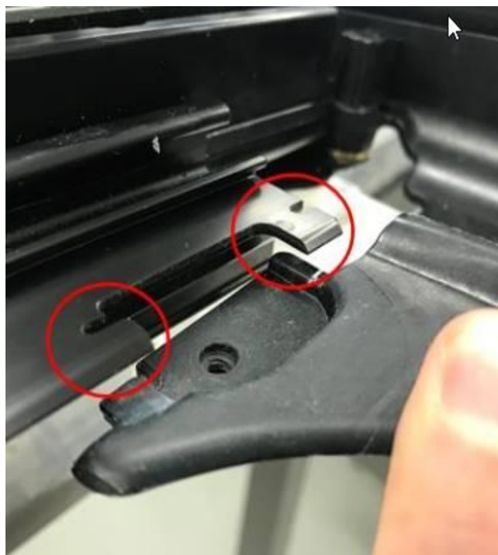
Figure 5. Removing the roller shade.
