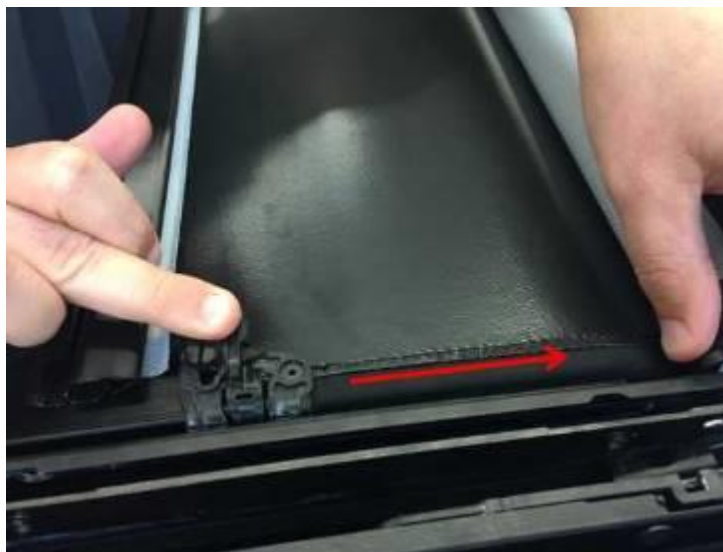
Figure 2. Loosening the roller shade.
