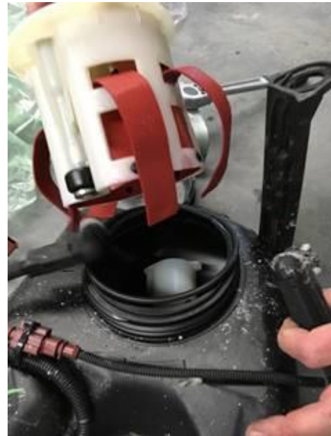
Figure 1. Filter element housing is loose inside the tank.
