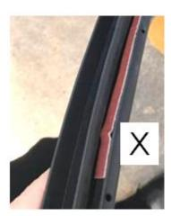
i. Repeat from step e to attach all of the adhesive tape (1) between the position marks.
