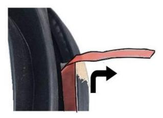
k. Clean the vehicle panel hemming part where the adhesive tape on the seaming welt will be attached.
