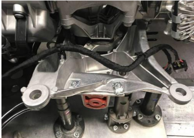
Figure 6. Routing and mounting of the transmission harness behind the crossmember.
