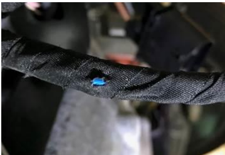
Figure 2. Example of a small rip in the protective tape.
