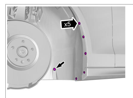
Remove the screws. Remove the clips.
