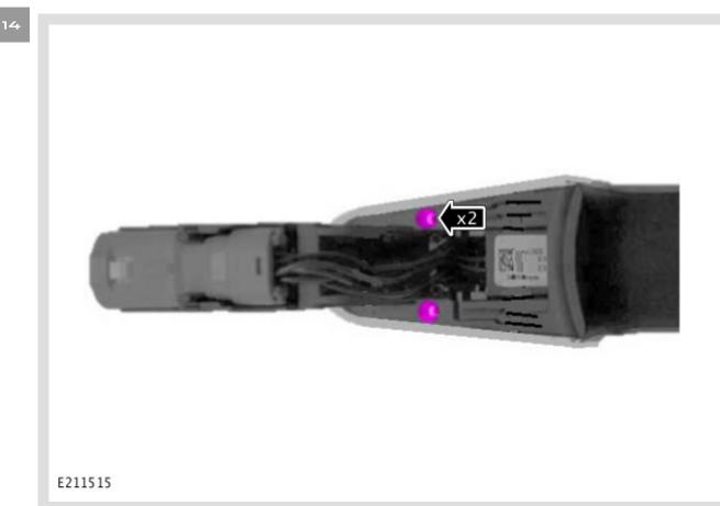
Install the 2 screws into the handle strap.
