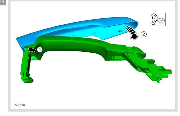
Assemble the inner and outer sections of the door exterior handle by clamping the 2 sections together.
