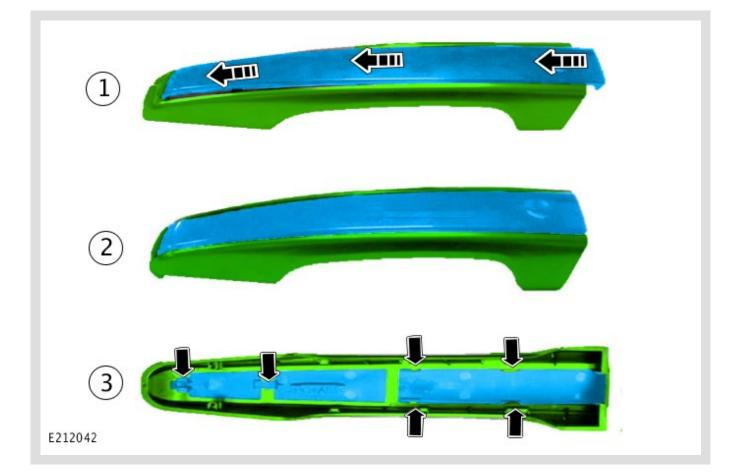
Install the painted door exterior handle insert into the door exterior handle cover (1).
