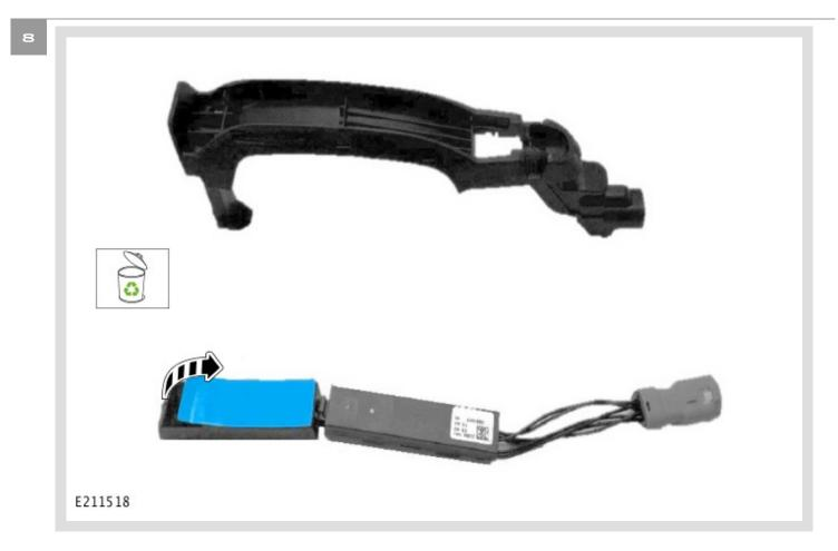
Prepare the door exterior handle strap inner and electronic module for assembly.
