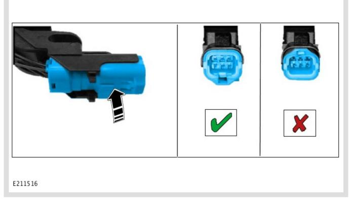
Clip the electrical connector into the handle strap inner ( $\checkmark$ ).
