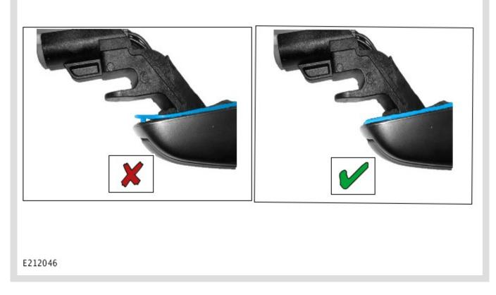
Make sure the rubber gasket sits flush against the handle base and the locating lug at the front of the gasket is installed into the hole in the handle ( $\checkmark$ ).
