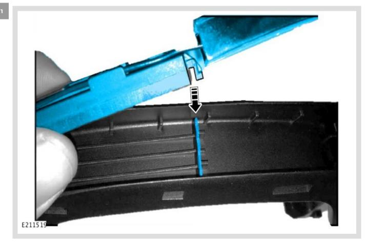
Install the antenna and electronic unit into the handle strap inner; align the clip with the handle strap inner rib.
