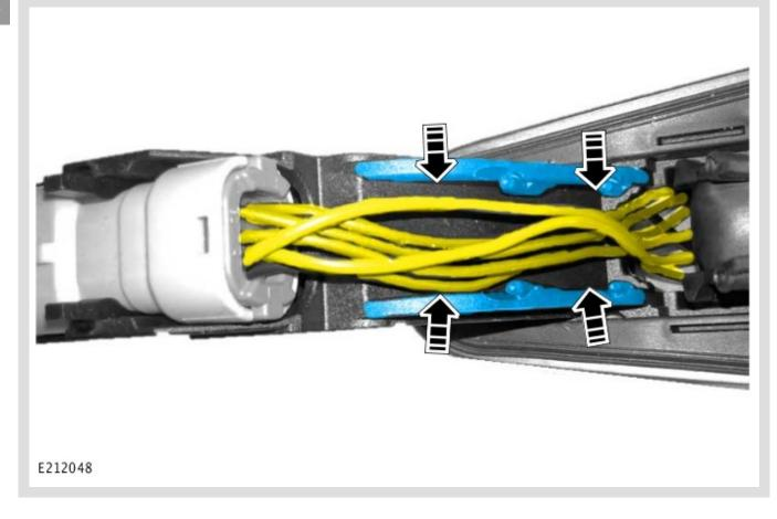
Make sure the wiring harness is positioned.
