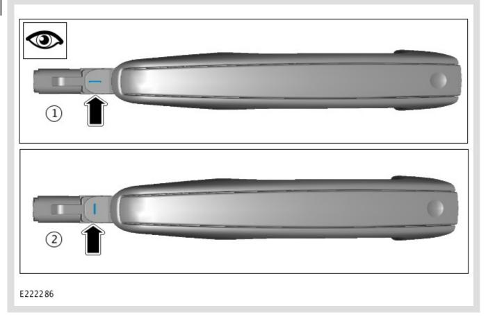
Inspect the marking(s) on the replacement door exterior handle(s).
