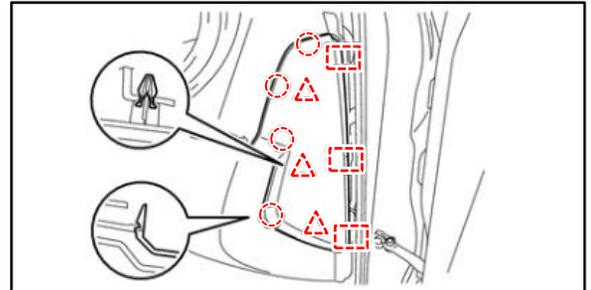
17. Remove the glove box compartment plate by disengaging the five clips.
