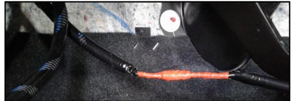
60. Repeat the same joint terminal wrapping process as used in steps 57 – 59, using electrical tape.
