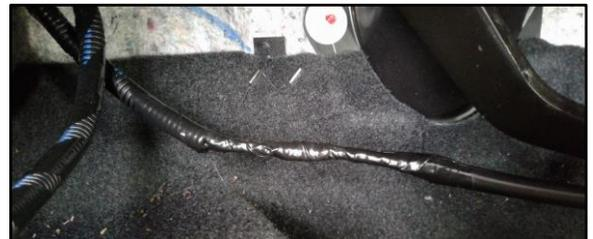
61. At the splice location on the NEW A/C ECU sub-wire harness, gently fold the A/C ECU sub-wire harness onto itself, join it with the NEW driver J/B sub-wire harness, wire-tie both harnesses to the I/P harness, and cut off the excess from the tie band.
