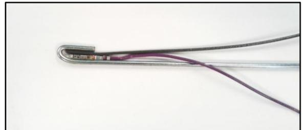
30. Using silicone tape, measure a 40 mm length, cut with scissors, and snugly wrap the bent end of the wire coat hanger and two wire ends with the silicon tape.
