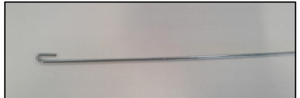
29. Place the ends of the driver J/B sub-wire harness and A/C ECU pigtail into the bent end of the coat hanger wire.
