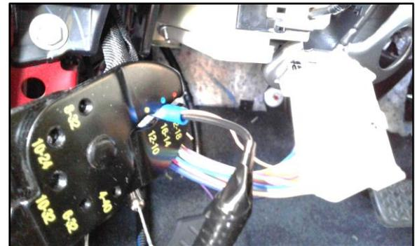
K. Squeeze the crimp tool until the ends of the crimp tool come in contact with each other, ensuring a good quality crimp.
