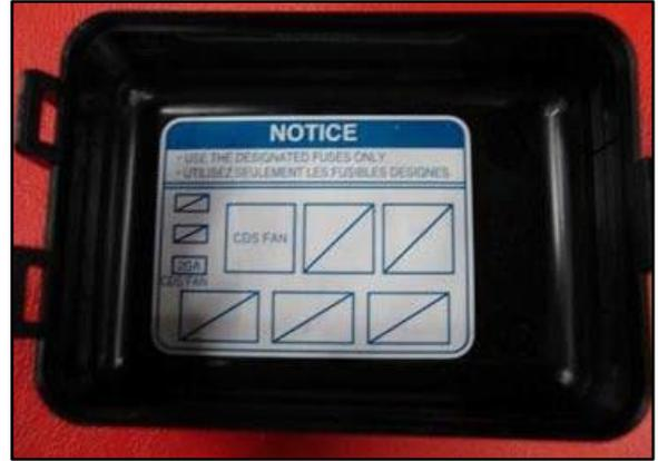
10. Install the NEW relay into the “CDS FAN” location as indicated on the notice label.
