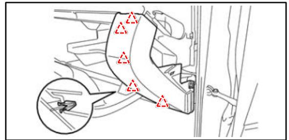
18. Remove the lower No. 2 instrument panel airbag assembly.
