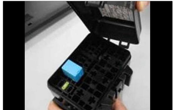
11. Attach the relay block to the bracket installed in step 8.
