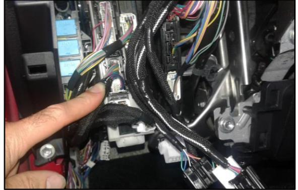
40. Remove the black, plastic lock lever from the connector.
