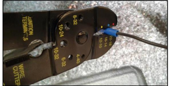
54. Squeeze the crimp tool until the ends of the crimp tool come in contact with each other, ensuring a good-quality crimp.
