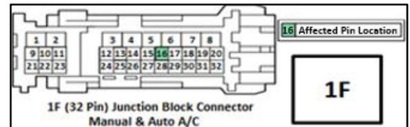
42. Confirm there is a pin and wire in pin location 16 in connector 1F. The connection will be made with a wire splice procedure.
