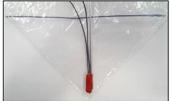
32. Wrap the bent end of the wire coat hanger with the cut corner of the plastic parts bag and dip the end in isopropyl rubbing alcohol.
