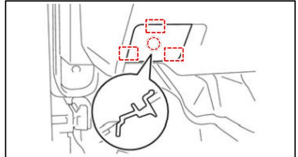
15. Remove the instrument panel lower finish panel sub-assembly.
