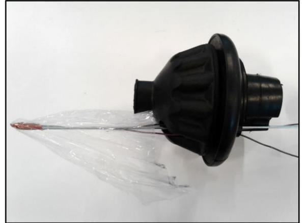
35. Gently remove the plastic and the silicone tape, taking care to not damage the wire ends, and free the wires from the wire coat hanger. Gently pull the remaining length of the wire coat hanger through the passage and discard.
