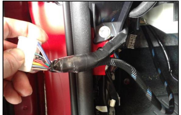
45. Reinstall the black plastic lock lever to connector 1F.
