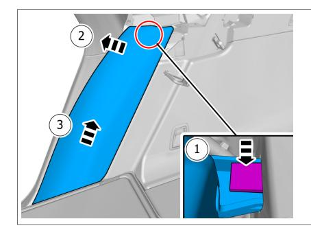
Release the catch. Remove the marked part.
