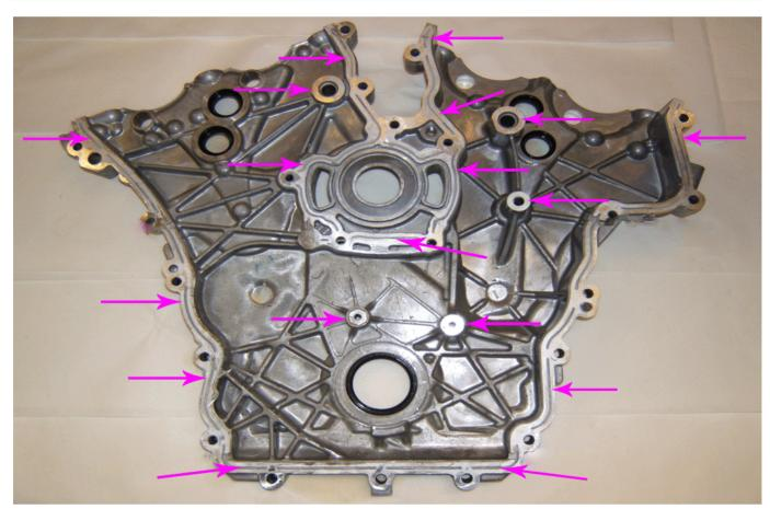
24. Apply a 3 mm bead of RTV sealant to the remaining front cover sealing surfaces.
