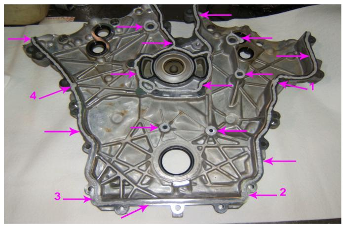
25. This is a typical view of the proper application of the RTV sealant to the front cover, with a 5 mm bead of RTV sealant to the T-joints (1, 2, 3, 4) and a 3 mm bead of RTV sealant to the rest of the sealing surfaces.
