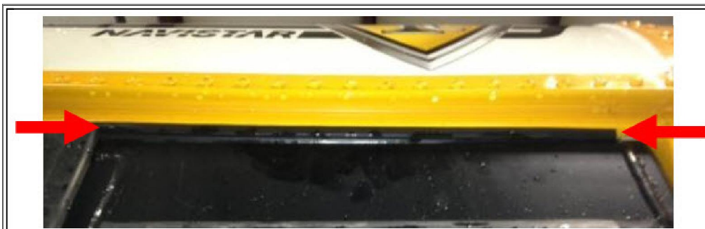
Upper Door Casing Seal Evenly Compressed
