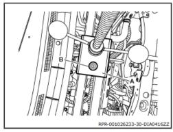
72. Tighten handle of Tool (A) to support the weight of the engine and transaxle assembly. Refer to Engine Support Tool Operating Instructions.
