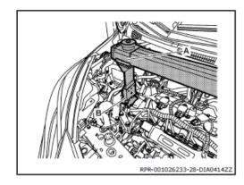
Install Tool (A) to Tool (C) as shown. Refer to Engine Support Tool Operating Instructions.
