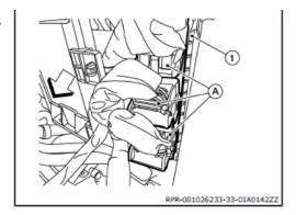
67. Using a suitable tool, release harness retainer (A) and position harness (1) aside.
