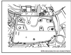
9. Remove nuts (A) and remove harness bracket (B) from battery tray (1).
