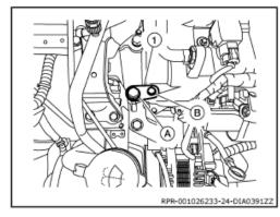
65. Install Tool (B) as shown with supplied bolt (C). Refer to Engine Support Tool Operating Instructions.
