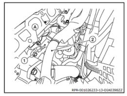
21. Disconnect the harness connector from the knock sensor. Refer to "Component Parts Location" in the Engine Control System section of the ESM.
