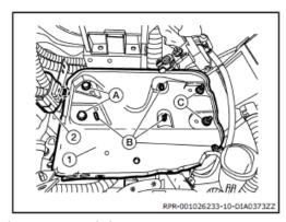
11. Release pawl and separate battery positive cable (2) from battery tray (1).
