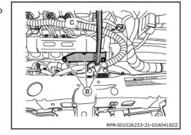
Install Tool (C) to rear of the engine using bolts (B) supplied with Tool. Refer to Engine Support Tool Operating Instructions.
