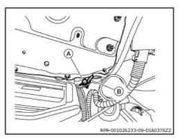
6. Remove TCM bolts and set TCM aside. Refer to "Exploded View" in the Transaxle and Transmission section of the ESM.
