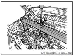
Using bubble level (B) on Tool (A) level Tool as shown.
