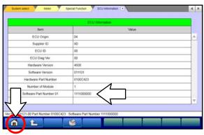
d. If the Software Part Number listed is **not** at the latest level (shown in the "Combination Meter Reprogramming Chart" in this TSB), proceed with the next step. Click the Home button to return to the System Select screen.
