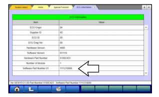
Confirm "Software Part Number" now matches the NEW one shown in the "Combination Meter Reprogramming Chart" in this TSB.
