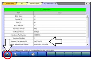
d. If the Software Part Number listed is **not** at the latest level (shown in the "Engine ECU Reprogramming Chart" in this TSB), proceed with the next step. Click the Home button to return to the System Select screen.
