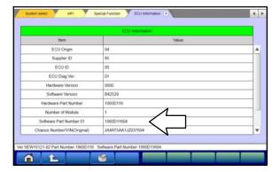
Confirm "Software Part Number" now matches the NEW one shown in the **"Engine ECU Reprogramming Chart"** in this TSB.
