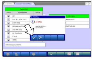
c. A window will pop up asking you to confirm DTC erasing. Click the check mark in the dialog box for DTC erasing and reading to begin.
