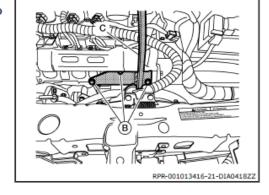
Install Tool (C) to rear of the engine using bolts (B) supplied with Tool. Refer to Engine Support Tool Operating Instructions.
