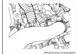
29. Using a suitable tool, release pawl and set harness (1) aside.
