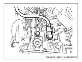
Disconnect the harness connector (A) from the transaxle assembly.
