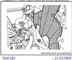
Install front portion of Tool (A) on driver's side frame rail (1) as shown. Refer to Engine Support Tool Operating Instructions.
