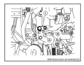
64. Install Tool (B) as shown with supplied bolt (C). Refer to Engine Support Tool Operating Instructions.
