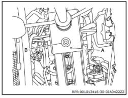
71. Tighten handle of Tool (A) to support the weight of the engine and transaxle assembly. Refer to Engine Support Tool Operating Instructions.
