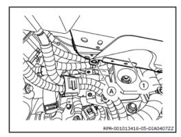
Disconnect the harness connector (A) from EVAP canister purge volume control solenoid valve.
