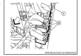
66. Using a suitable tool, release harness retainer (A) and position harness (1) aside.
