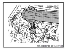
69. Install Tool (A) to Tool (C) as shown. Refer to Engine Support Tool Operating Instructions.
