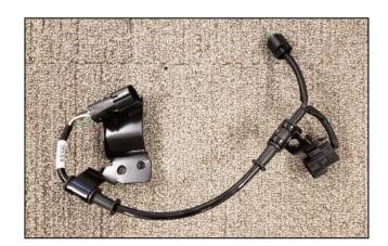
6. Install the new ECS extension harness in reverse order of removal.
