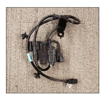
6. Install the new ECS extension harness in reverse order of removal.
