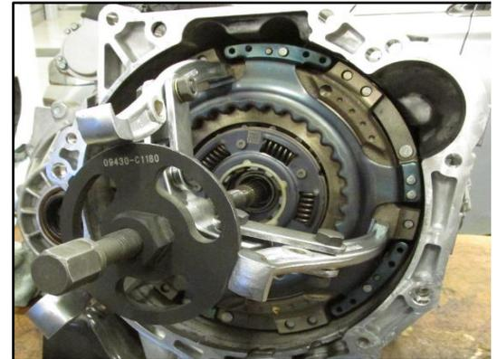
5. Remove the 2 bolts (D) securing the fork cover. Remove the 6 bolts (E) retaining the clutch actuator assembly to the transmission.
