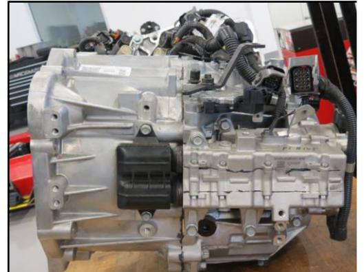
9. Install the new Double-Clutch using the special service tool (SST 09430-2A240) to fully seat the Double-Clutch.
