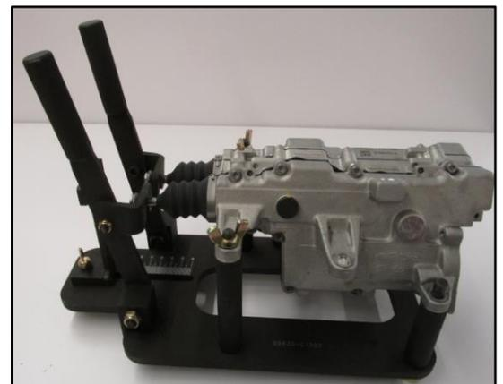
7. Follow the service shop manual procedure to initialize the rod length for both odd and even clutch actuator rods.
