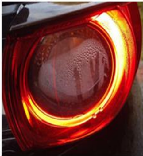
CONDENSATION RUNNING DOWN LENS - REPLACE LIGHT UNIT
