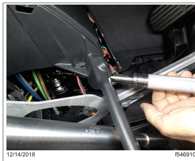
Fig. 3, Tightening the Brake Light Pressure Switch
