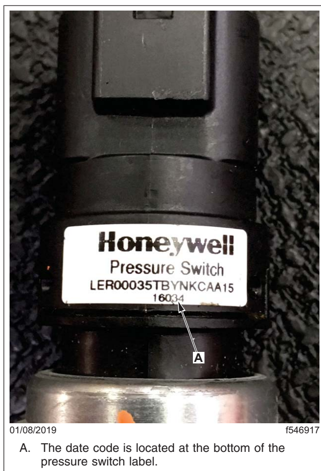
Fig. 2, Brake Light Pressure Switch Date Code
