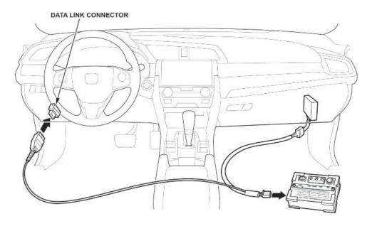
5.6. Turn the power switch to **ON**. A solid green LED should come on.
