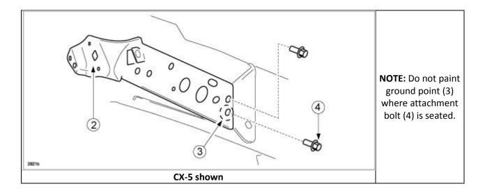
Customers concern can be resolved by sanding off paint at ground point (3) where attachment bolt (4) is seated. After installing the bolt (4), apply touch-up paint to the exposed base material area of the front fender stay.
