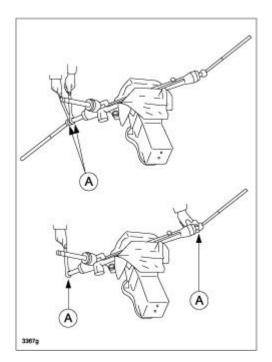
5. Install the driver side spacer (A) and passenger side spacer (B) onto the steering rack bar as shown below.
