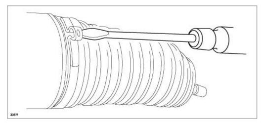
c) Remove the boot from the steering gear.
