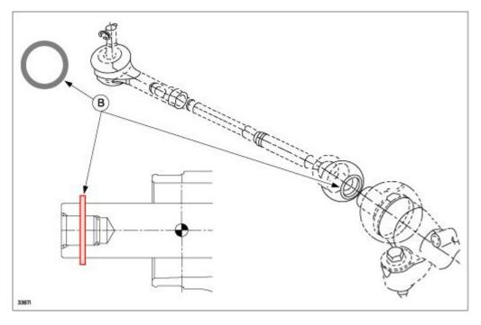
6. Install the tie rod assembly (both sides) according to the instructions on MGSS online:
