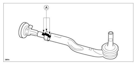
b) Insert a flathead screwdriver into the boot band (as shown below), then press the caulked area outward to remove the boot band (both sides).
