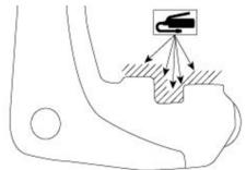
• Apply a thin coating of brake grease to the ends of the new brake pads where they contact the pad clips.
