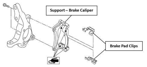
• Before installing new brake pads, remove the pad clips and **thoroughly** clean the caliper support of any dirt, rust or corrosion, paying close attention to the areas where the clips are attached / seated.
