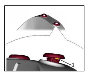
Realign the seat cover to the seatback frame and reinstall the headrest guides, ensuring that the release buttons <1> are fully seated.
