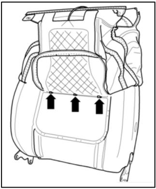
Fold the cover up and pry the cover profile out of the cushion mounts <arrows> using a small screwdriver (or equivalent).
