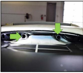
Release the retainers <arrows> securing the headrest guides to the seat frame and push the guides towards the top of the seat to remove them.
