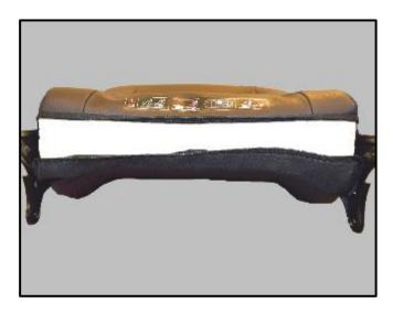
Roll the cover downwards and fold over the seatback bottom <as shown>.
