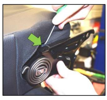
Using a small screwdriver (or equivalent) extract the end of the seatback zipper on both sides of the seat <arrow>.
