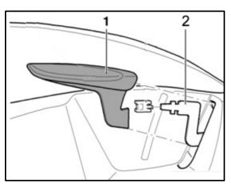
• If equipped, reinstall the adjustment handle <1> to the adjusting lever <2>.
