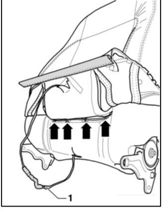
Fold the cover further down and install the new upholstery clamps <arrows> using Upholstery Clip Pliers - VAG1634 (or equivalent).
