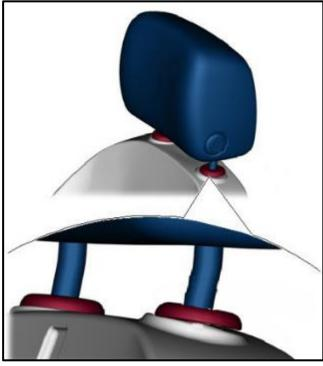
Reinstall the headrest to the seat, ensuring it is fully seated.
