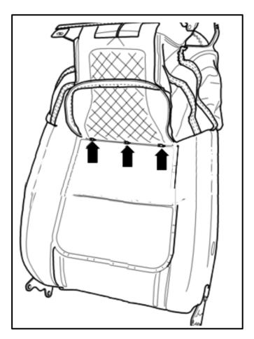
• Fold the cover down and reattach the cover to the cushion mounts <arrows>.
