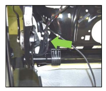
Release any remaining wiring harness retainers located in the area near the seatback hinge <arrow>.
