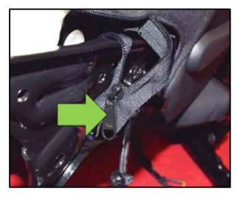
• Install the slide <arrow> - P/N 1S0881451 to the seatback cover zipper.
