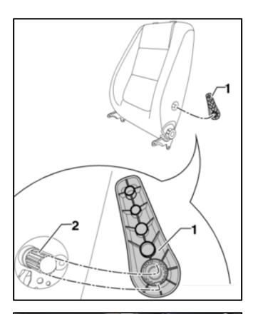
• If equipped, reinstall the lumbar adjustment lever <1> onto the shaft <2>, ensuring the splines in the lumbar adjustment lever align with the splines on the shaft.
