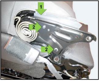
Remove the seatback trim plates <arrow 1> on both sides of the seat by releasing the retainers <arrow 2> then using a Pry Lever 80-200 (or equivalent) to remove the trim plate.
