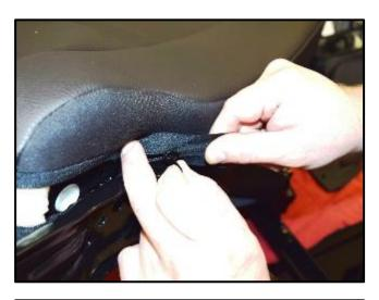
Using the slide, zip the seatback cover completely until the slide detaches itself from the other end of the zipper.
