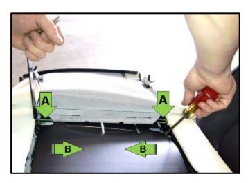
Fold the cover up and remove the rear cover mount rod <arrow A> by using a pair of Pry Levers 80-200 (or equivalent) to gently compress the lumbar adjustment frame in the direction shown <arrow B>.
