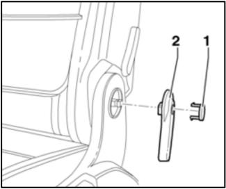
• If equipped, reinstall the release lever <2> and then the release lever cap <1>.
