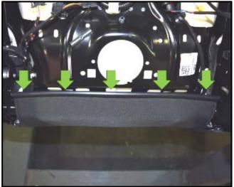
• Reattach the lower seat cover channel to the seat bottom pan <arrows>.
