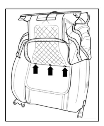
• Fold the cover down and reattach the cover to the cushion mounts <arrows>.
