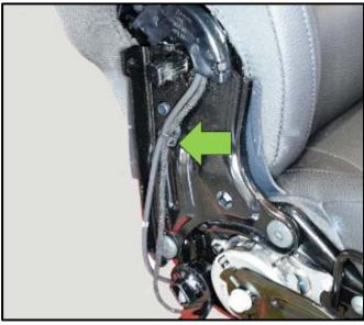
Carefully remove the seat and airbag wiring harnesses from the seatback frame.
