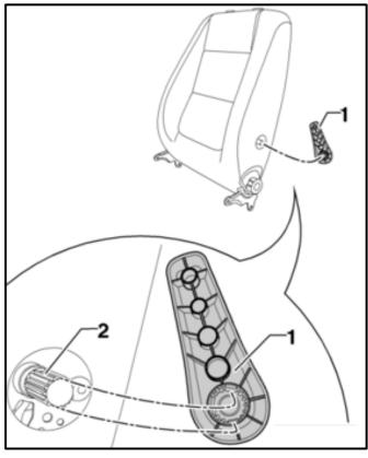
If equipped, pull outward on the lumbar adjustment lever <1> and remove it from the shaft <2>.
