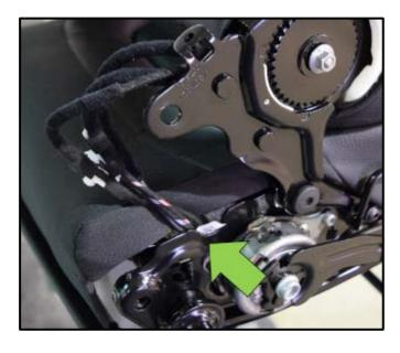
• Carefully remove the seat and airbag wiring harnesses from the seat bottom <arrow>.
