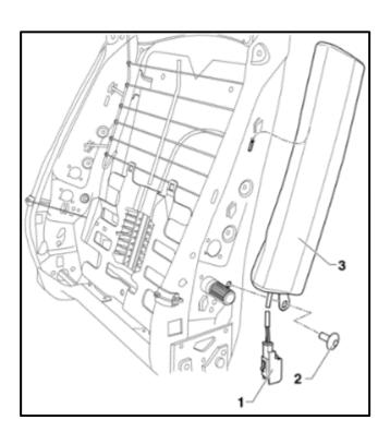
• Install the replacement side airbag <3> to the mount in the backrest frame.
