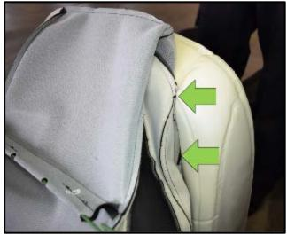
Install new upholstery clamps <arrows> on both sides of the seat using Upholstery Clip Pliers - VAG1634 (or equivalent).
