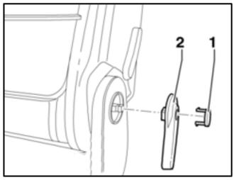
• If equipped, remove the release lever cap <1> and remove the release lever <2>.
