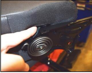
Once zipping the seatback cover has been completed, tuck the end of the zipper into the seat <as shown>.
