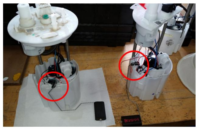
The picture below is a cut away of the right fuel module indicating the level sender contacting the side of the fuel tank.
