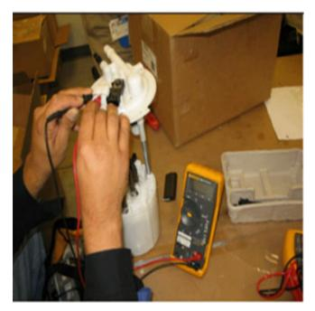
When testing the sweep of the fuel level sensor, slowly sweep the float arm from the empty position to the full position watching the ohm meter looking for a momentary O.L. or open reading. You should see the sweep range from approximately 40 ohms to 250 ohms, + or - 5 ohms.
