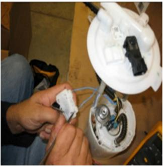
Once sensor is removed from assembly carefully depress lock tabs on both sides of the sensor to remove the terminals from the fuel level sensor assembly.
