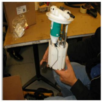
Note: Do not remove the fuel level sensor from the fuel module unless you get a faulty reading during the testing of the sensor. This may cause damage to the fuel level sensor unnecessarily.
