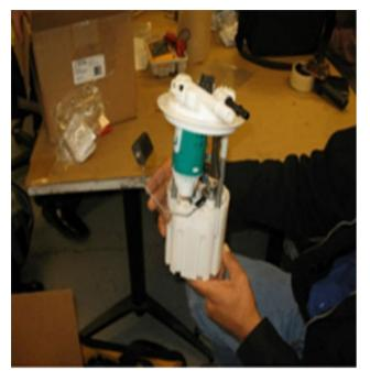
Upon a successful sweep test, reinstall module into the fuel tank, reassemble the components and verify successful repair.
