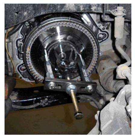
Important: To install bearing use Special Tools DT-22928-B Seal Installer per SI, as damage may occur if the proper tools are not utilized. Proper bearing orientation is the writing up or visible to technician.
