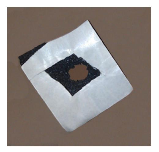
6. Add two ¾" by 1 1/2 " long by 7/16" thick of Kent Adhesive Backed Shim Stock (foam) p/n P46505 or equivalent centered between the retaining clips on the leading edge of the package shelf (behind/under the rear seat back) see picture below.
