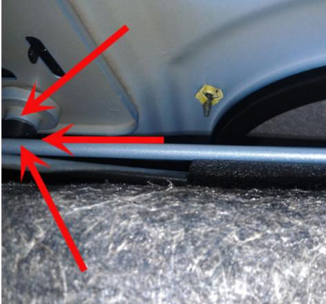
4. Add felt onto the package shelf trim opening to prevent movement between the trim and the child seat tether cover if the felt is not present. Use Kent Adhesive Backed Flocking Tape p/n KT13295 or equivalent see pictures below.
