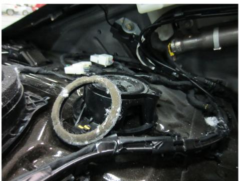
2. OnStar module - place 1/4" foam pad underneath the module (if foam is not currently in place). Use (4) 1" x 6"x 5/16" thick strips of Kent Adhesive Backed Shim Stock (foam) p/n P46510 or equivalent.
