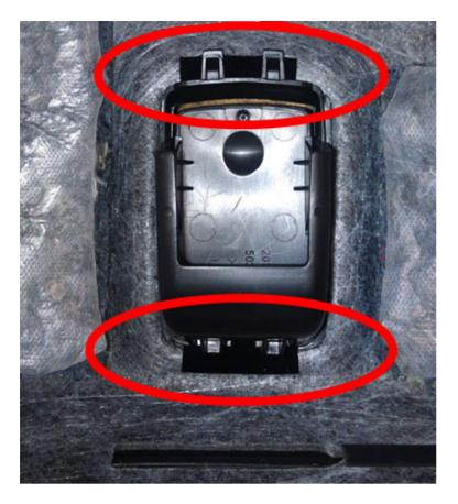
5. Add foam grommets onto each of the Christmas tree fasteners (if not present) prior to reinstalling back into the package shelf sheet metal holes. Use 1" X 1" block of Kent Adhesive Backed Shim Stock p/n P46510 or equivalent to create a foam washer(s) as needed. Fold the 1" x1" block over from corner to corner and carefully cut a hole in the center of the block to create a washer/spacer, see pictures below.
