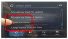
• Confirm the current Software Version ID. If the Current Version is **Rel\_UO.18.43.20**, **STOP** as this latest update has already been installed. Otherwise, proceed to **Step 2** below.
