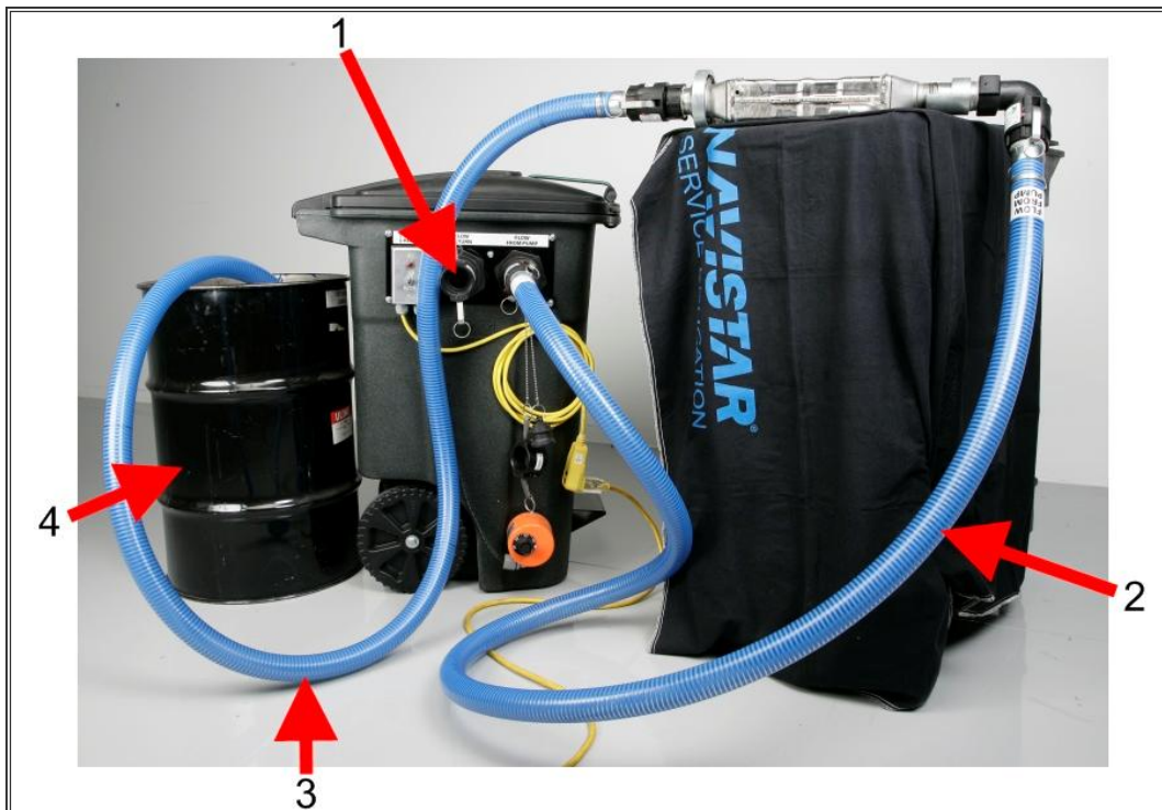
Figure 17. Draining Cleaning Management System (12-353-01A)
