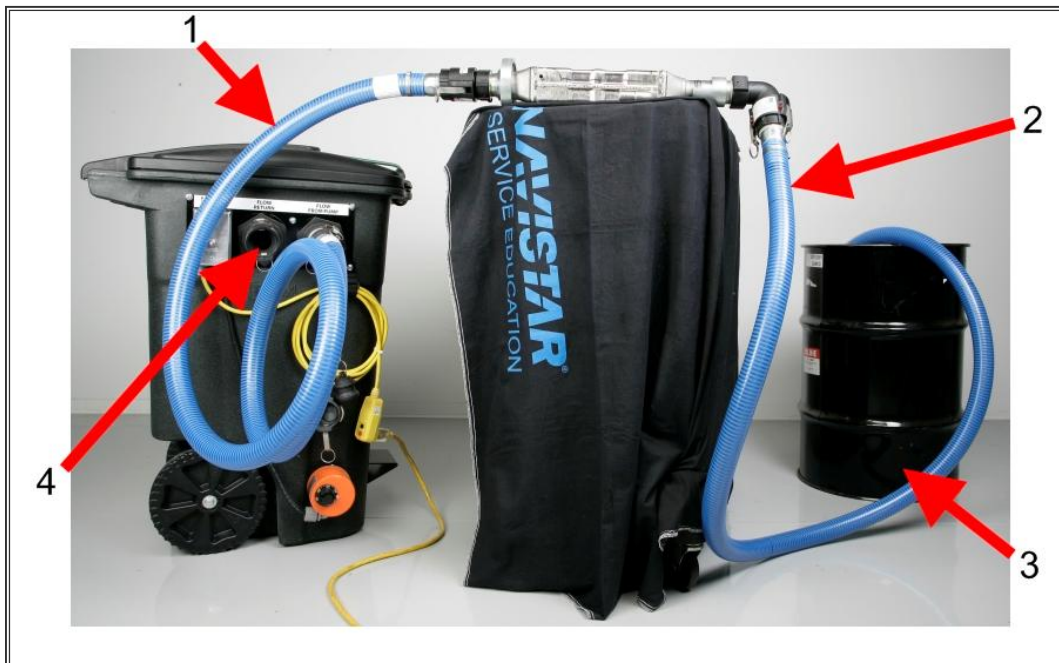
Figure 19. Draining Cleaning Management System (12-353-01A)
