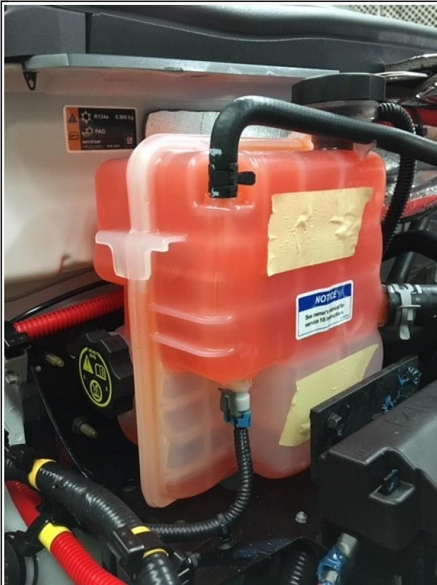
Proper fill with upper chamber full to top of tank (brim full) and residual coolant in lower chamber
