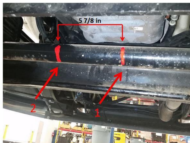
Figure 3: Tie rod assembly
