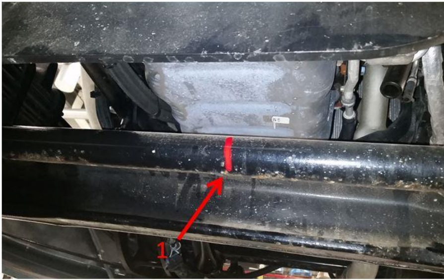
Figure 1: Tie rod assembly
