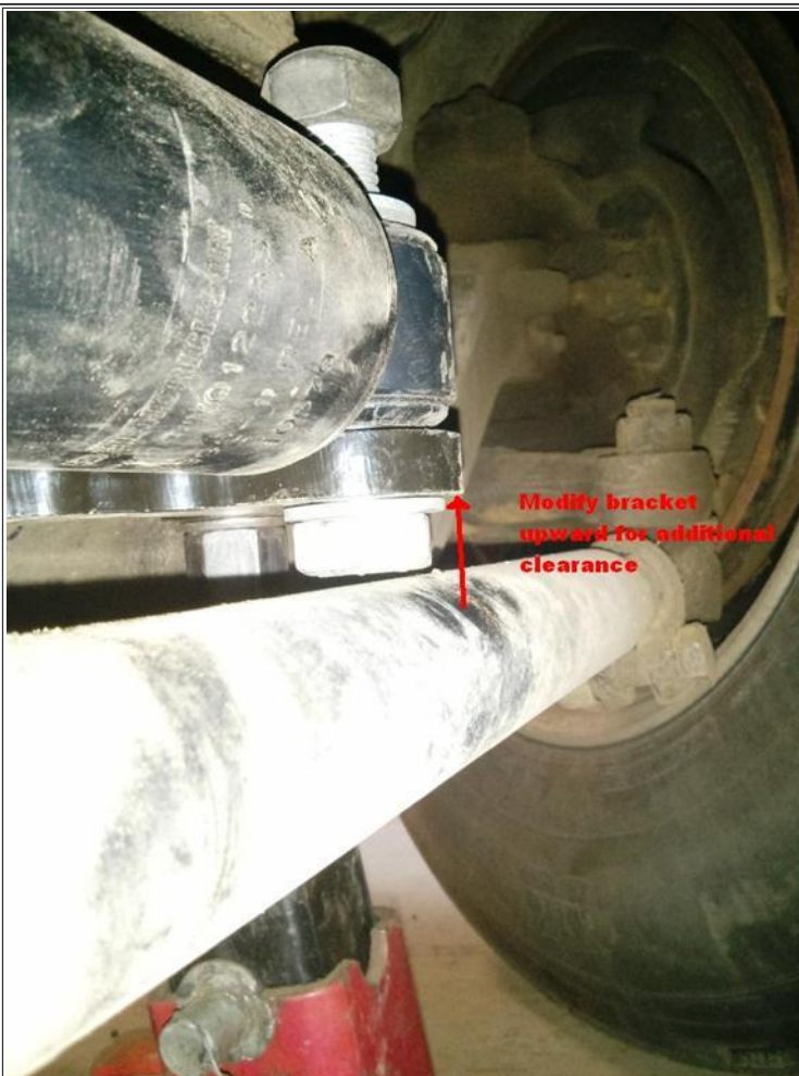
Figure 4: Tie rod tube to mount clearance
