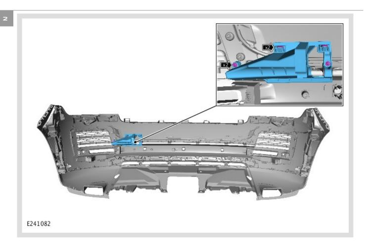
Remove and discard the front bumper blanking plate.
