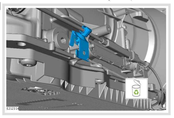
Remove and discard the  $\underline{\mathtt{EPB}}$  cable rear mounting bracket.
