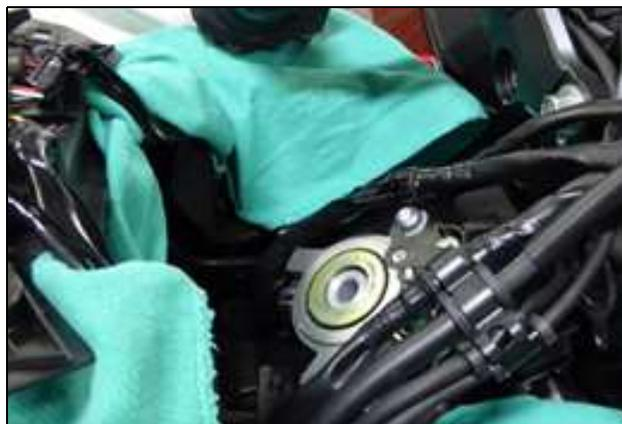
2. Clean the upper and lower bearing races then apply the specified grease to each steering bearing and dust seal lip.
