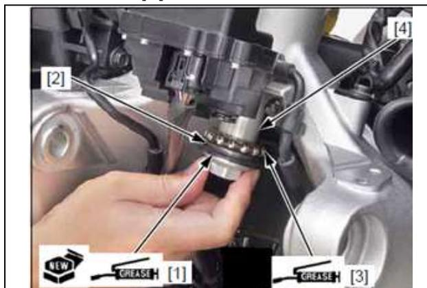
4. Insert the stem shaft into the steering head pipe then install the following parts while holding the stem shaft from below:
