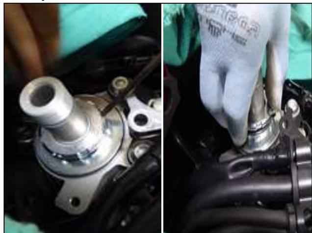
**Checkpoint:** How to determine if the stem shaft is damaged.
