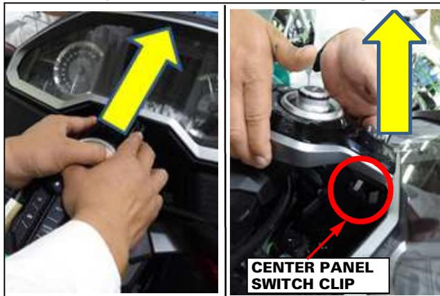
9. Remove the screws [1] from the top bridge cover [2]. Disengage the cover by lifting the rear of it then disengaging the front. Rotate center panel switch backwards, resting it on a clean towel. Note how cables and hoses are routed in the cover for re-assembly.
