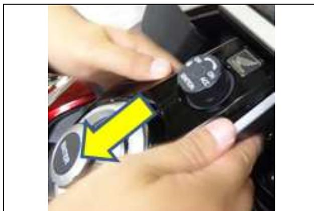
13. Lift the end of the top shelter and install the socket bolts for the center panel switch (left and right sides, two total).
