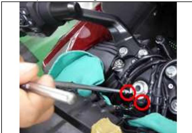
11. Remove the left rear handlebar bolt and washer [1].
