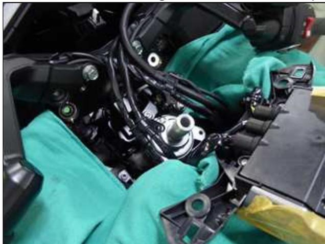
20. Flatten the tabs of the lock washer and remove the lock nut, the lock washer, and adjuster nut.
