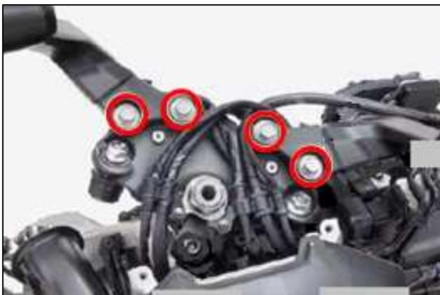
9. Install the cable clamps and cable clamp bolts then tighten each bolt to the specified torque below (left and right sides, two total).
