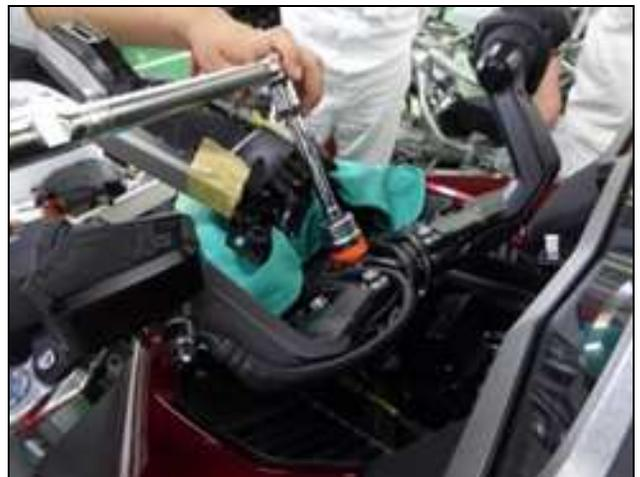
19. Lift the top bridge and handlebars as an assembly and rotate backwards while moving it towards the meter assembly.
