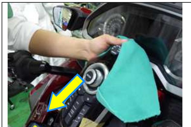
12. With the center panel switch moved forward, insert the clip at the front part of the center panel switch. Slide the center panel switch toward the rear of the motorcycle.
