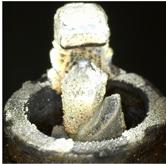
No good: Insulator badly broken
