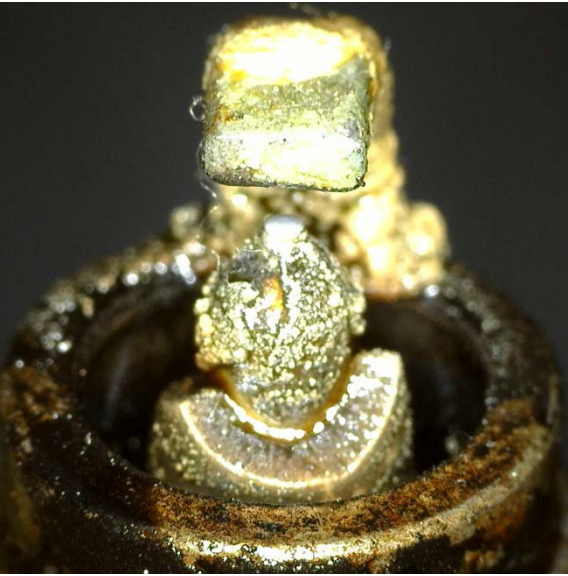
No good: Insulator badly broken
