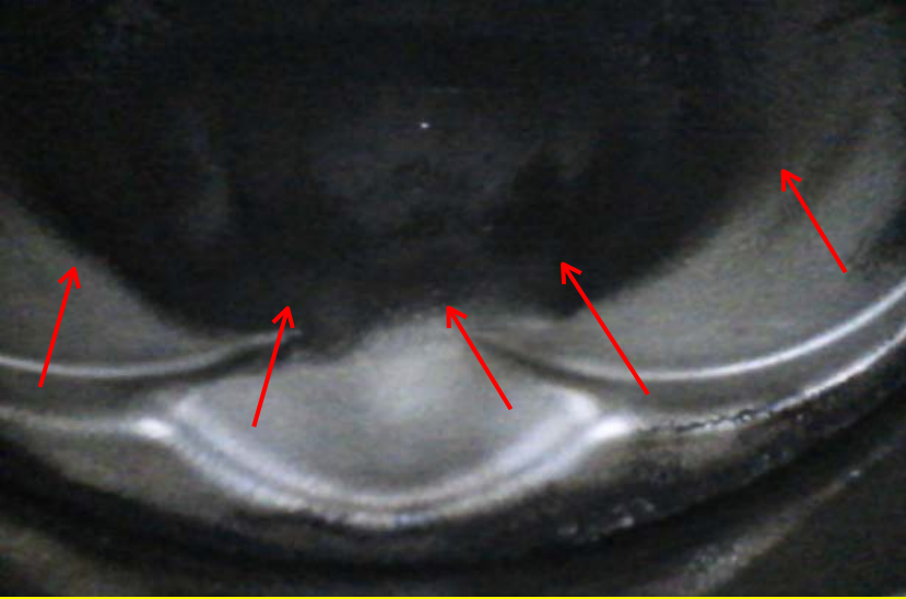
Good: A close up of a 2014 3.5L V6 (direct injection) with 60,000 miles and no oil problems. No oily deposits, just dry carbon and clean area on piston top from direct injection spray pattern.
