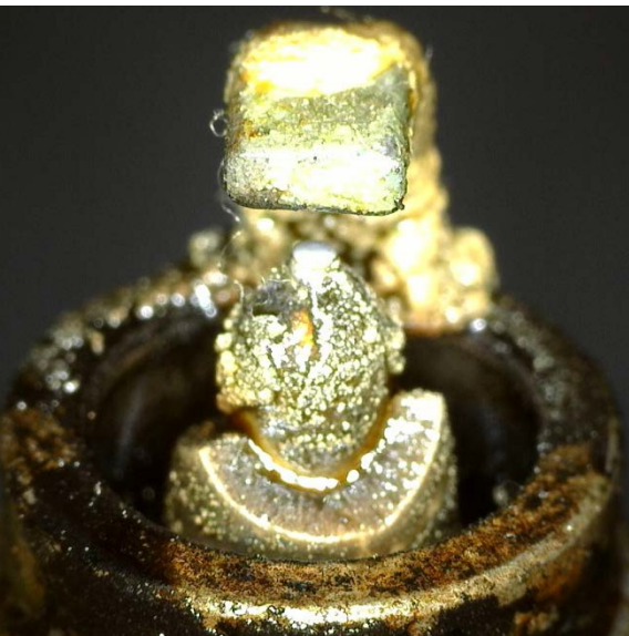
No good: Insulator badly broken
