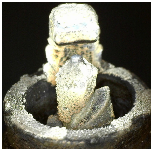
No good: Insulator badly broken
