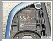
MEMS sensor in the remote key transmitter version 2.1. Remote keys can be differentiated between version 2.1 and the earlier version 2 by removing the back cover. Carefully check the ID printed in various places (circled). G05 basic remote key shown; other models similar.
