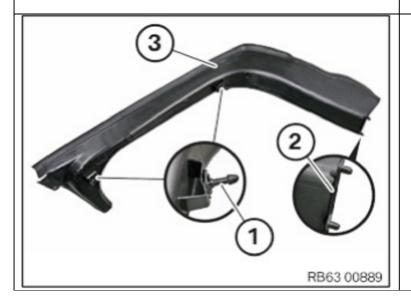
6. Check the clips (1) and guides (2) on the water channels for damage. If water channel clips are damaged, the water channel must be replaced.
