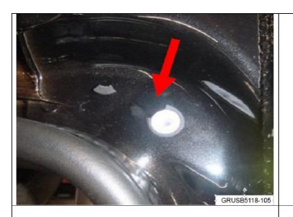
4. With both water channels removed, inspect the foam sealing rings of all 4 retaining clips for damage.
