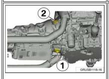
5. If the lower transmission housing also has oil residue present then it has to be cleaned via the opening (1). To do so, remove the sealing cap (1) and sealing cap (2) and flush out the excess engine oil residue. The sealing cap (2) may be located on the left or the right side of the transmission housing.
