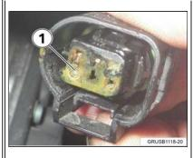
for traces of water or corrosion.
