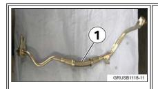
1. Stainless steel flexible section. This is the new design and should not be replaced.
