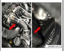
2. Check the exhaust turbocharger oil feed line on bank 1.
