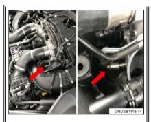
renew the oil feed line for the exhaust turbocharger N63O2" Do not remove the turbochargers!
