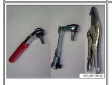
4. Use a suitable tool to hold the T30 side of the band clamp fastener.
