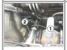
5. Hold the T30 stationary (1) and torque the 10 mm nut (2) to 8.5 Nm.
