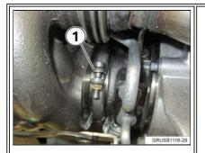
3. Remove the air filter box and locate the band clamp fastener (1).
