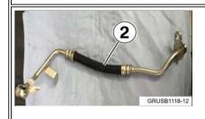
2. Black rubber flexible section. This line should be replaced.
