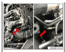
If the flexible section is black rubber then the oil feed line will need to be replaced.
