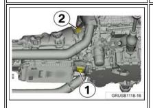
5. If the lower transmission housing also has oil residue present then it has to be cleaned via the opening (1). To do so, remove the sealing cap (1) and sealing cap (2) and flush out the excess engine oil residue. The sealing cap (2) may be located on the left or the right side of the transmission housing.
