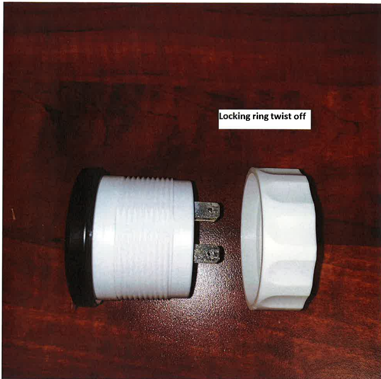
Pic 3. Showing the ring that removes from back of gauge to allow it to come out.
