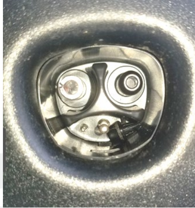
Figure 5 (Dislodged charge port insulator pin at lower right)
