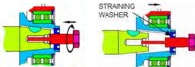
PULL OFF THE ROTOR WITH TOOL #680888 (shown)
