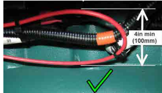
LTD is not a flexible harness. Avoid tight bends and kinks which could short circuit the LTD. Loops must have a minimum radii of 4 inches (100 mm)
