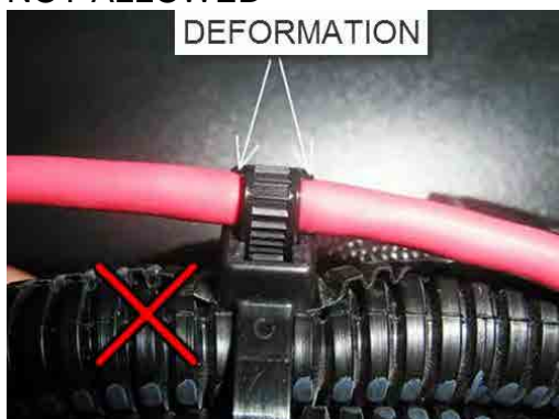
Cable tie tighten in excess on the LTD. Tighten cable tie on LTD by hand only. Tighten just enough to prevent LTD from slipping from once side to the other inside the cable tie loop
