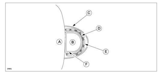
NOTE: Ensure the aluminum foil tape (F) is inserted into the edges of the molding (B) as shown below.
