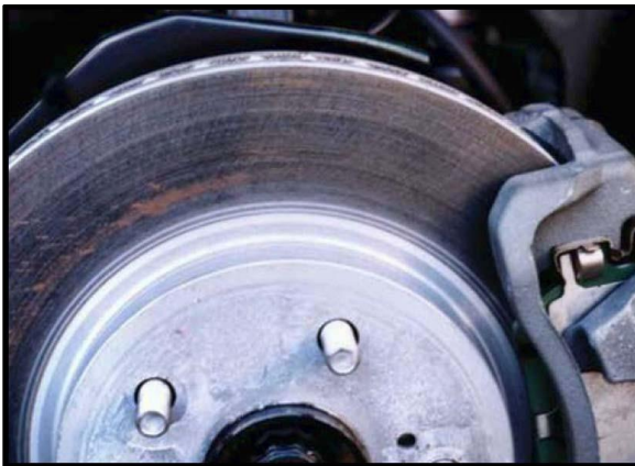
Figure 1. Slight Rust on Rotor (Easy to Remove by Braking)
