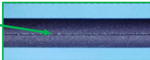
Using a metallic tool could result in damage to other components
