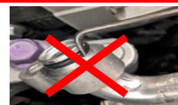
Using a metallic tool could result in damage to other components
