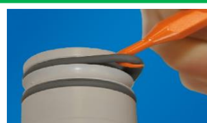
Use a non-metallic tool for O-ring removal.
