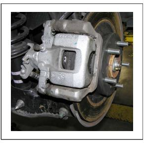
Reassemble the brake pad assembly, using the torque specifications from the applicable vehicle's Service Manual.
