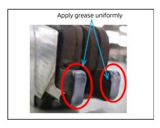
!! IMPORTANT!! Apply grease uniformly so that the base of the brake pads are completely covered with grease, as shown.
