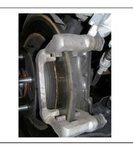
2. Clean the brake pad assembly and the clip mounting area of the caliper support with a brush.
